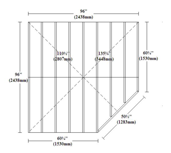
NB:- Floor joists run from right hand back to left hand front.
